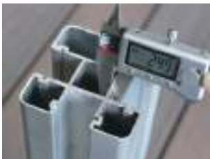
Post wall thickness 2.2-2.5mm
