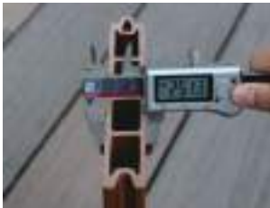
Fence board thickness 25mm
